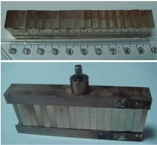
FIG. 7 (color online). Top: The pendulum is cut into 19 blocks to investigate the inhomogeneity of the coating layer. Bottom: The 19 blocks are assembled and the lateral (large) surfaces are coated.
