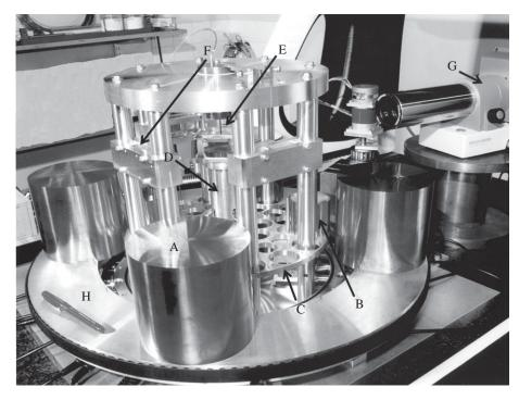
**Figure 1.** The Mk I apparatus: (A) one of the four source masses ( $\approx$ 11 kg); (B) one of the four test masses ( $\approx$ 1.2 kg); (C) the torsion disc about 30 cm in diameter; (D) the central tower holding mirrors, down the centre of which is suspended the torsion strip, just visible; (F) one of the three mirror supports part of the  $\times$ 6 multiplying optics; (G) the autocollimator; and (H) the carousel.
