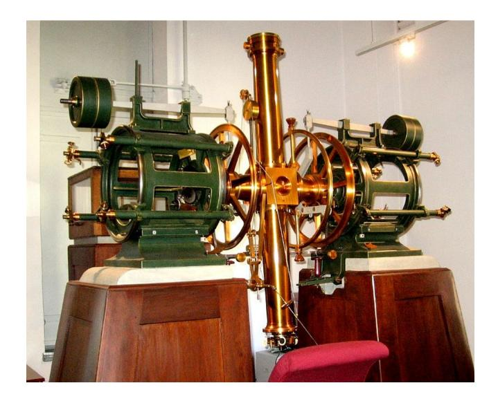
Meridian circle at the <u>Kuffner observatory</u>, Vienna, Austria, built by Repsold & Sons, Hamburg, 1886. Note the counterweights, the short, green cylindrical objects at the outer top of the mechanism, and the four long, thin, microscopes for reading the circles.
